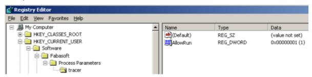
The setting in this example allows loading an executable from a file with the base name "tracer". The base name comparison is case-insensitive.
