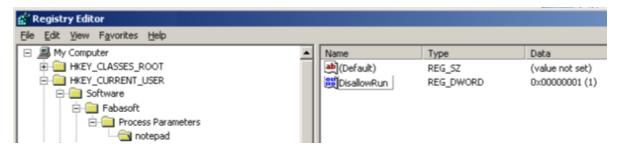
The setting in this example does not allow loading any executable from a file with the base name "notepad". The base name comparison is case-insensitive.
