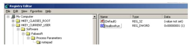
The setting in this example does not allow loading any executable from a file with the base name "notepad". The base name comparison is case-insensitive.
