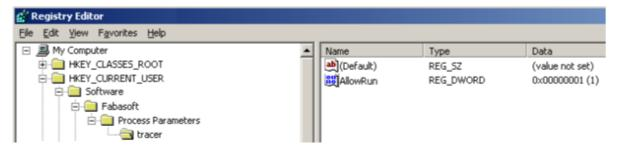
The setting in this example allows loading an executable from a file with the base name "tracer". The base name comparison is case-insensitive.
